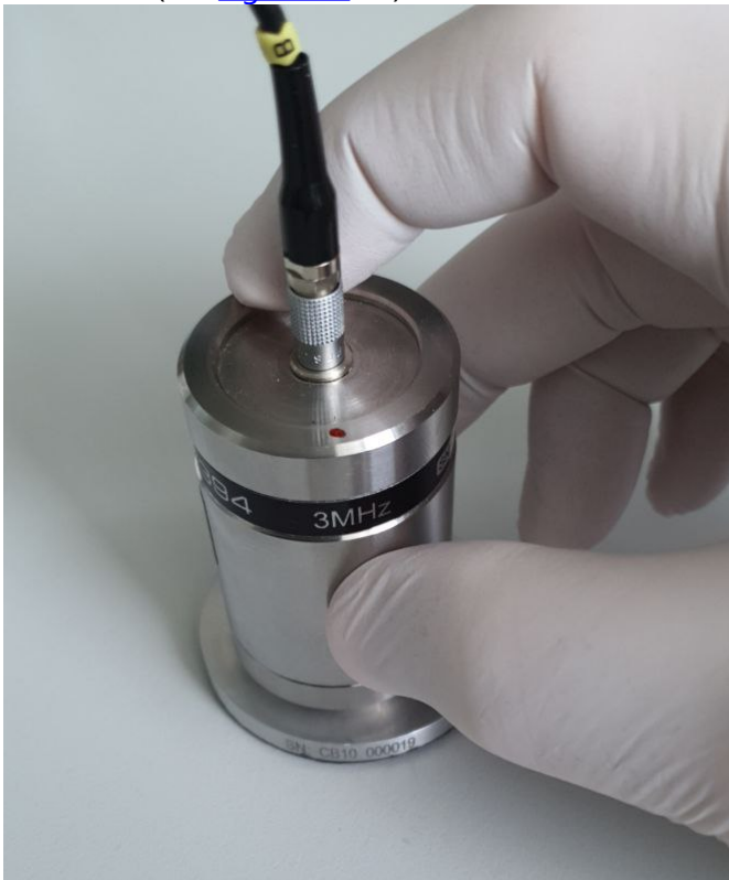
Figure 13: Calibrate device on calibration sample
