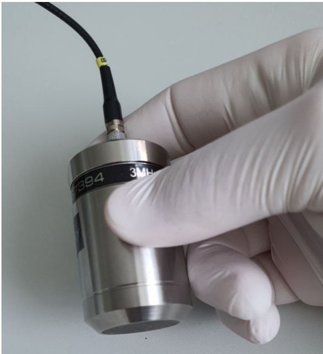
Figure 12: Calibrate probe in air
